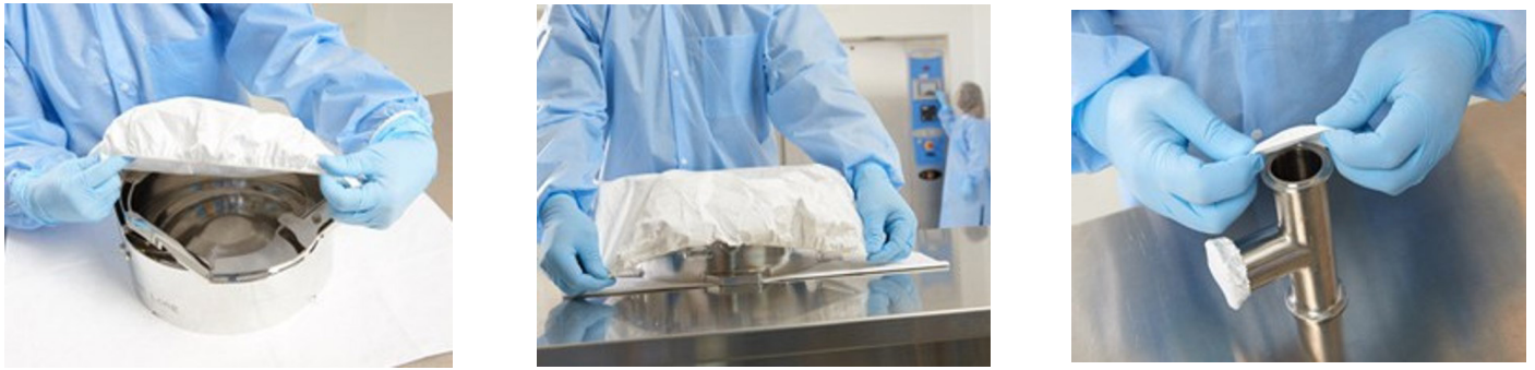
Figure 1. To apply an elasticized cover, stretch it over the opening, then pull the sides downward
